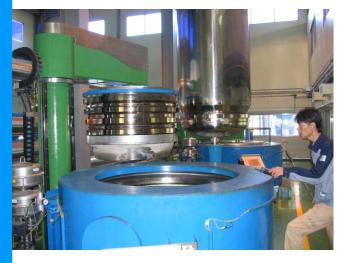
Special equipment design for edible oil production was implemented in this plant in Korea, which has an extractor volume of 2x3,8 m<sup>3</sup> and is one of the biggest worldwide designed for a pressure of 550 bar. It is an example of large-scale supercritical fluid extraction for products with a limited margin for production costs.
