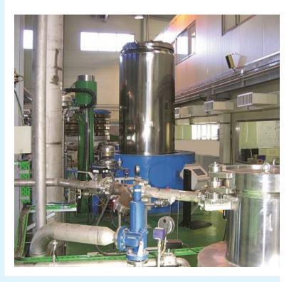
SFE also shows advantages for extraction of wood oils, because the process is strongly diffusion controlled and temperatures are lower compared to steam distillation.
